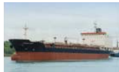
mt Pembroke Fisher – modern double-hulled tanker operated by James Fisher and Sons.
